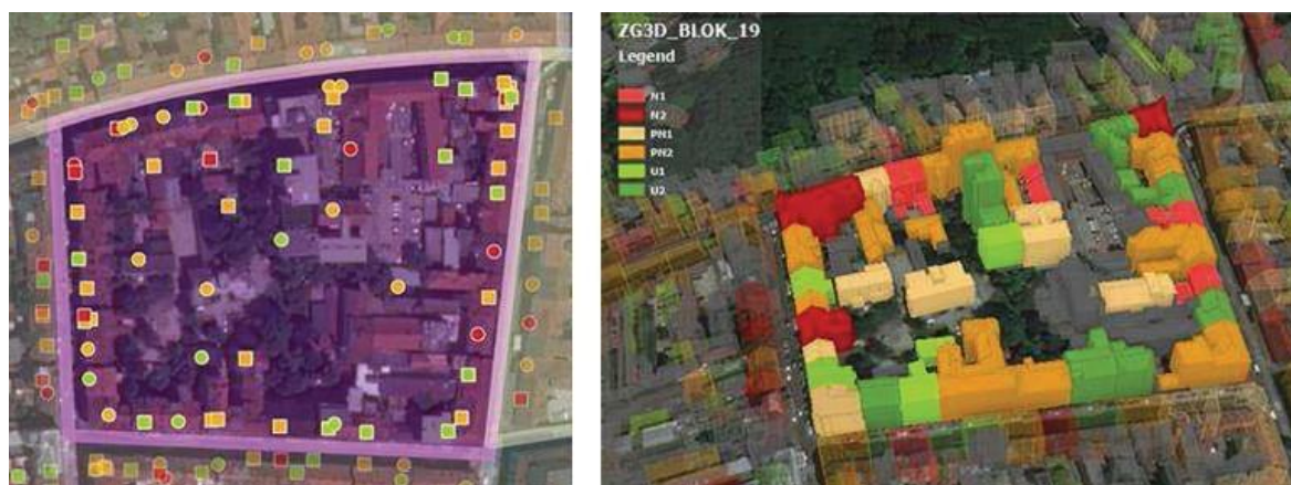
Fig. 5: Assessment of usability of buildings in Block_19 after the Zagreb earthquake; Structural Models of Renewal (part of the comprehensive renewal of the protected Historic Urban Core of the City of Zagreb – Lower Town); Source: Faculty of Civil Engineering, University of Zagreb, Zagreb, 2021.
